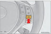
3 Press and hold the "DISP" button after selecting the desired setting item by pressing the "DISP" button.
