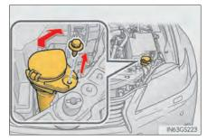
**2** Turn the bulb base counter-clockwise.
