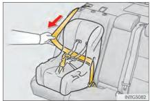
For While pushing the child restraint system into the rear seat, allow the shoulder belt to retract until the child restraint system is securely in place.
