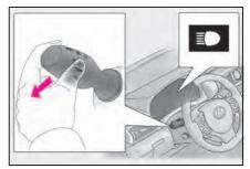
2 Press the Automatic High Beam switch.
