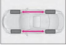
To equalize tire wear and extend tire life. Lexus recommends that tire rotation is carried out at the same interval as tire inspec-
