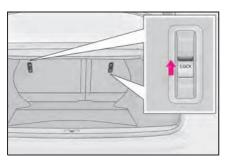
To lock a luggage security system lever from inside the cabin, fold the rear seatback forward, move the lever to the lock position, and return the seatback to its original position.
