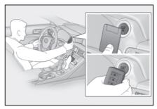
When the electronic key is detected, a buzzer sounds and the engine switch will turn to IGNITION ON mode.
