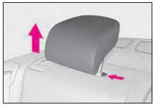
2 Flip up and fold the cover, and fix it with the hook-and-loop fastener.
