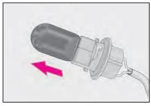
7 Install a new light bulb then install the bulb base to the light unit by inserting it and turning the bulb base clockwise.
