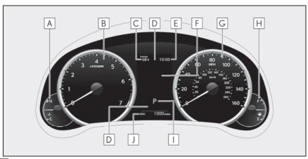
A Engine coolant temperature gauge
