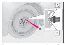
When replacing an aluminum wheel with an aluminum wheel, turn the wheel nuts until the washers **A** come into contact with the disc wheel **B**.
