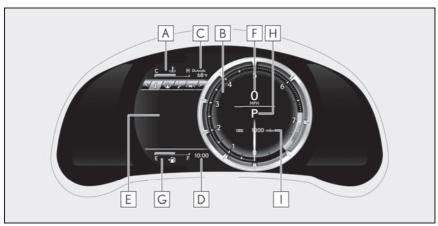
A Engine coolant temperature gauge
