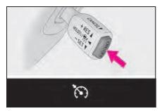
Accelerate or decelerate, with accelerator pedal operation, to the desired vehicle speed (at or above approximately 25 mph [40 km/h]) and push the lever down to set the speed.
