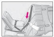
While pushing the child restraint system down into the rear seat,
