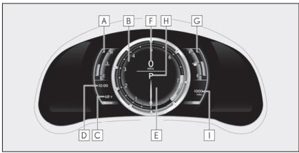
A Engine coolant temperature gauge
