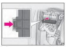
► Engine compartment: type B fuse box
