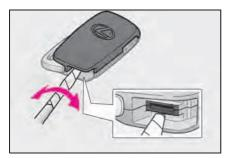
3 Remove the depleted battery.
