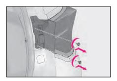
4 Pull the light unit toward the rear of the vehicle to remove it.
