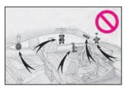
Do not hang coat hangers or hard objects on the coat hooks. All of these items could become projectiles and may cause death or serious injury, should the SRS curtain shield airbags deploy.
