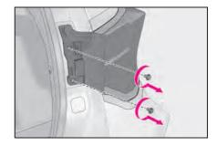
4 Pull the light unit toward the rear of the vehicle to remove it.
