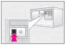
3 Press and hold the desired HomeLink<sup>®</sup> button (inside the vehicle) for 2 seconds and release it. Repeat this sequence (press/hold/release) up to 3 times to complete programming. If the garage door opener motor operates when the HomeLink<sup>®</sup> button is pressed, the garage door opener motor recognizes the HomeLink<sup>®</sup> signal.
