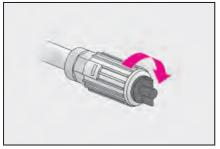
If the air release cap is not attached, the sealant may leak and the vehicle may get dirty.
