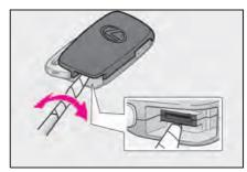
**3** Remove the depleted battery.
