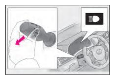
2 Press the Automatic High Beam switch.
