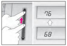
The temperature setting can also be adjusted by touching on the sensor.
