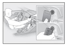
When the electronic key is detected, a buzzer sounds and the engine switch will turn to IGNITION ON mode.
