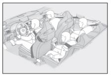
The pretensioners help the seat belts to quickly restrain the occupants by retracting the seat belts when the vehicle is subjected to certain types of severe frontal collision or a vehicle rollover.
