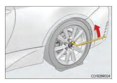
3 Turn the tire jack portion "A" by hand until the notch of the jack is in contact with the jack point.
