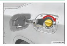
2 Close the fuel filler door, and press the center of the rear edge of the fuel filler door until you hear a click. When you lock the doors, the fuel filler door will also lock.
