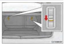
2 Pull the seatback lock release lever and fold the seatback down.
