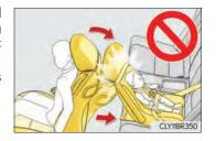
• Do not allow the child to lean his/her head or any part of his/her body against the door or the area of the seat, rear pillars or roof side rails from which the SRS curtain shield airbag deploys even if the child is seated in the child restraint system. It is dangerous if the SRS curtain shield airbag inflates, and the impact could cause death or serious injury to the child.
