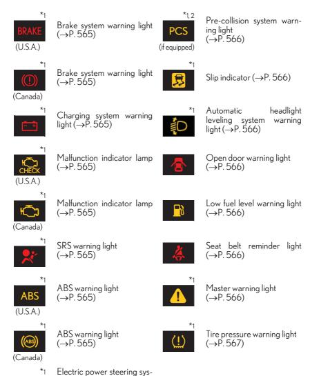
\*1: These lights turn on when the engine switch is turned to IGNITION ON mode to indicate that a system check is being performed. They will turn off after the engine is started, or after a few seconds. There may be a malfunction in a system if a light does not come on, or turn off. Have the vehicle inspected by your Lexus dealer.
