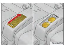
Rear cup holder insert can be removed.
