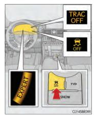
■ When the message is displayed on the multi-information display showing that TRAC has been disabled even if has not been pressed (RC350/RC300)
