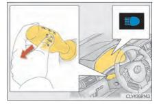
2 Press the Automatic High Beam switch.
