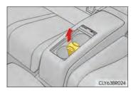
• The rubber mats at the bottom of the front cup holders can be removed.
