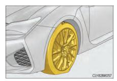
• To avoid sealant leakage, move the vehicle until the area of the puncture, if known, is positioned at the top of the tire.
