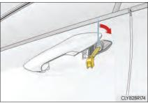
Remove the key, return the handle, and then pull the handle again.
