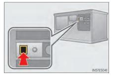
HomeLink button (inside the vehicle) for 2 seconds and release it. Repeat this sequence (press/hold/release) up to 3 times to complete programming. If the garage door opener motor operates when the HomeLink button is pressed, the garage door opener motor recognizes the HomeLink signal.
