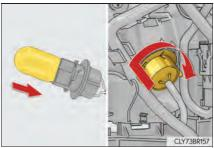
**5** Align the tabs and push the light unit toward the front of the vehicle to install it.
