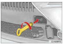
Tighten down the towing eyelet securely using a wheel nut wrench or hard metal bar.
