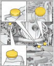
RC F: While the engine and radiator are hot, do not loosen or remove the coolant reservoir cap.
