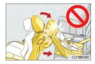
• Do not allow the child to lean his/her head or any part of his/her body against the door or the area of the seat, rear pillars or roof side rails from which the SRS curtain shield airbag deploys even if the child is seated in the child restraint system. It is dangerous if the SRS curtain shield airbag inflates, and the impact could cause death or serious injury to the child.
