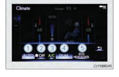
If the "A/C" indicator is turned off, the system will blow ambient temperature air or heated air.
