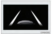
Indicates that the system is recognizing white (yellow) lines. When the vehicle departs from its lane, the white line displayed on the side the vehicle departs from flashes orange.
