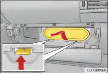
4 Press the tabs and remove the filter case.
