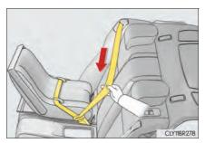
Shile pushing the child restraint system down into the rear seat, allow the shoulder belt to retract until the child restraint system is securely in place.
