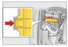
▶ Engine compartment: type B fuse box
