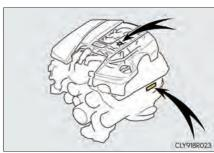
The engine number is located as shown.
