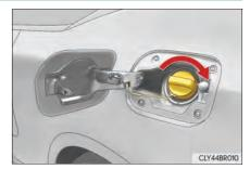
Close the fuel filler door, and press the center of the rear edge of the fuel filler door until you hear a click. When you lock the doors, the fuel filler door will also lock.
