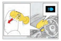
2 Press the Automatic High Beam switch.
