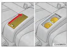
Rear cup holder insert can be removed.
