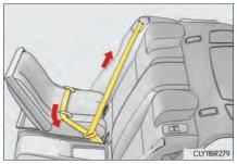
6 After installing the child restraint system, rock it back and forth to ensure that it is installed securely.
