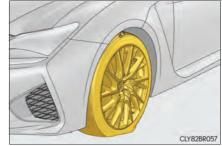
• To avoid sealant leakage, move the vehicle until the area of the puncture, if known, is positioned at the top of the tire.
