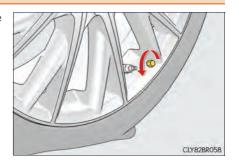
**2** Extend the hose. Remove the air release cap from the hose.
