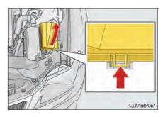
► Driver's side instrument panel Remove the lid.
