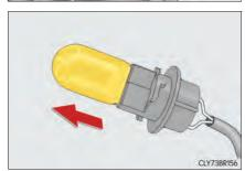
Install a new light bulb then install the bulb base to the light unit by inserting it and turning the bulb base clockwise.
