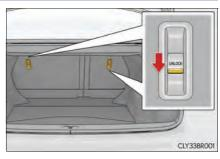
2 Pull the seatback lock release lever and fold the seatback down.
