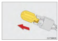
4 Install a new light bulb then install the bulb base to the light unit by inserting it and turning the bulb base clockwise.
