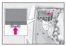
► Engine compartment: type B fuse box (LC500h)
