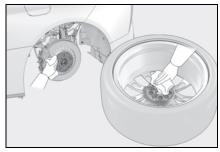
Install the tire and loosely tighten each wheel nut by hand by approximately the same amount. Turn the wheel nuts until the washers come into contact with the disc wheel.
