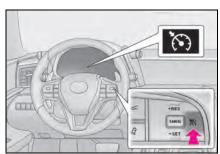
Accelerate or decelerate, with accelerator pedal operation, to the desired vehicle speed (at or above approximately 25 mph [40 km/h]) and press the "-SET" switch to set the speed. Cruise control "SET" indicator will come
