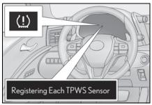
6 Drive the vehicle at 25mph (40 km/h) or more for approximately 10 to 30 minutes.
