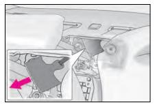
LC500h: Using the tab to open the fuel filler door may not allow for an adequate reduction in fuel tank pressure before refueling. To prevent fuel from spilling out, turn the cap slowly when removing it.
