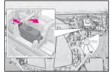
4 Connect a positive jumper cable clamp to A on your vehicle and connect the clamp on the other end of the positive cable to B on the second vehicle.
