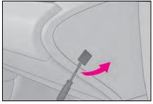
Push the flathead screwdriver into the part shown in the illustration to open the glove box.
