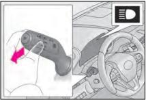
2 Press the Automatic High Beam switch.
