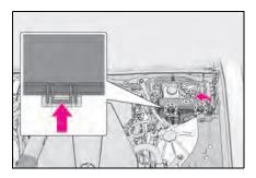
► Engine compartment: type C fuse box (LC500h)
