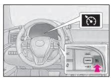
2 Accelerate or decelerate, with accelerator pedal operation, to the desired vehicle speed (at or above approximately 25 mph [40 km/h]) and press the "-SET" switch to set the speed.
