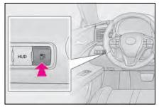
Open the fuel filler door until it is securely locked.
