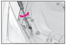
**2** Turn bolt B in either direction as step **1**.
