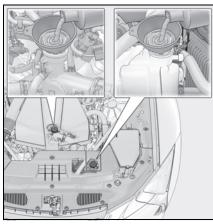
Start the hybrid system and turn the air conditioning system on to check that the radiator cooling fan operates and to check for coolant leaks from the radiator or hoses.
