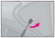
2 Push the flathead screwdriver into the part shown in the illustration to open the glove box.
