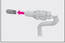
Install a new light bulb and then install the bulb base to the light unit by inserting it and turning it clockwise.
