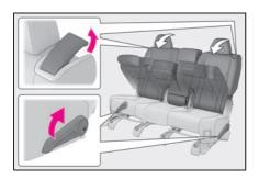
2 Pull the seatback folding lever and fold the seatback.
