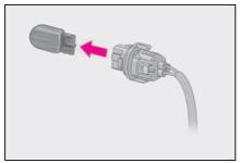
5 Install a new light bulb and then install the bulb base to the light unit by inserting it and turning it clockwise.
