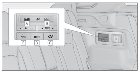
A Adjust the rear seats fan speed setting
