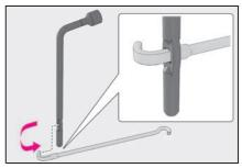
5 Connect the jack handle to the adapter socket. Turn the jack handle counterclockwise.
