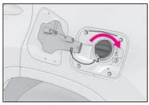
Close the fuel filler door, and press the center of the rear edge of the fuel filler door.
