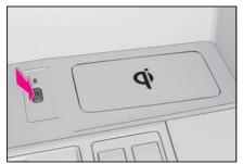
Place a portable device on the charging area with its charging surface facing down.
