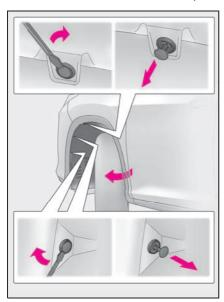
2 Pull back the fender liner until the connector is visible.
