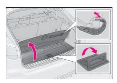
2 Attach the hook to the upper edge of the back door opening as shown.
