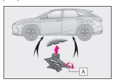
4 Raise the vehicle until the tire is slightly raised off the ground.
