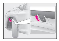
3 Partially remove the fender liner and turn the bulb base counterclockwise and remove it.
