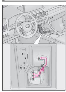
While the engine switch is in IGNI-TION ON mode, move the shift lever with the brake pedal depressed.
