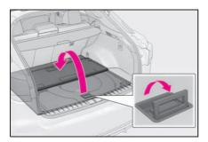
2 Lift the deck board and disengage the hook on the underside of the deck board.
