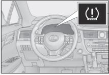
7 Drive the vehicle at approximately 25 mph (40 km/h) or more for approximately 10 to 30 minutes until the inflation pressure of each tire is displayed on the multi-information display.
