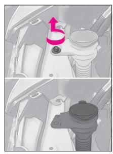
3 Turn the bulb base counterclockwise and remove it.
