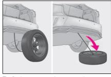
5 Before raising the tire, make sure that the hoist assembly is perpendicular to the wheel opening. (Try to place the tire directly beneath the vehicle, near where the wire cable is hanging from.)
