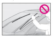
Do not operate the wiper lever when the windshield wipers are lifted. Otherwise, the windshield wipers may contact the hood, possibly resulting in damage to the windshield wipers and/or hood.
