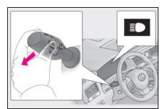
2 Press the Automatic High Beam switch.
