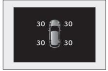
If the tire pressure drops below a predetermined level, the driver is warned by a screen display and a warning light. (
