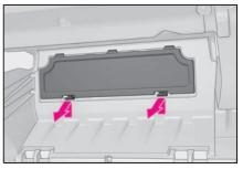
5 Unlock the filter cover (A), pull the filter cover out of the claws (B), and remove the filter cover.
