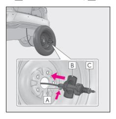
**8** Tilt the bracket **B** and pass it through the wheel opening. Then remove the hoist assembly **C**.
