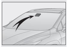
If the system judges that the vehicle is being driven over the speed limit, performing prohibited actions, etc. in relation to the recognized road signs, it notifies the driver using a notification display and notification buzzer.
