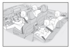
The pretensioners help the seat belts to quickly restrain the occupants by retracting the seat belts when the vehicle is subjected to certain types of severe frontal or side collision or a vehicle rollover.
