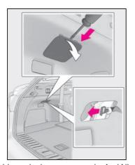
Using the lever to open the fuel filler door may not allow for an adequate reduction in fuel tank pressure before refueling. To prevent fuel from spilling out, turn the cap slowly when removing it.
