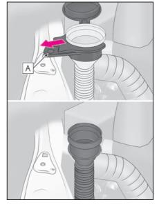
4 Turn the bulb base counterclockwise and remove it.
