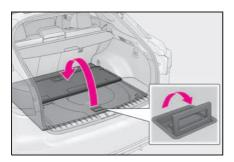
2 Lift the deck board and disengage the hook on the underside of the deck board.
