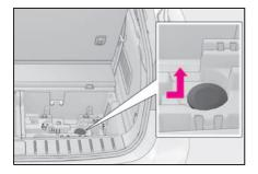
**3** Attach the adapter socket to the spare tire clamp bolt.
