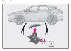
4 Raise the vehicle until the tire is slightly raised off the ground.
