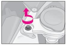
**3** For the right side only: Open the cap, remove the bracket **A**, and move the washer fluid inlet.
