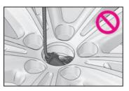
If the spare tire clamp bolt is turned without a tire on the hoist assembly, the wire cable may not be able to be lowered. If the wire cable cannot be lowered, contact your Lexus dealer.
