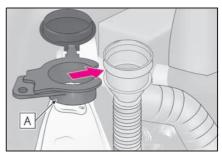
8 For the right side only: Fix the washer fluid inlet.
