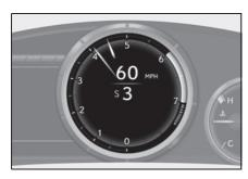
■ The meters and display illuminate when The power switch is in ON mode.
