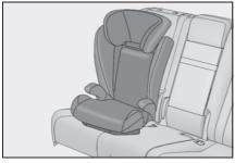
4 Sit the child in the child restraint system. Fit the seat belt to the child restraint system according to the manufacturer's instructions and insert the plate into the buckle. Make sure that the belt is not twisted. Check that the shoulder belt is correctly positioned over the child's shoulder and that the lap belt is as low as possible.  $(\rightarrow P.26)$
