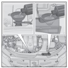
Start the hybrid system and turn the air conditioning system on to check that the radiator cooling fans operate and to check for coolant leaks from the radiator or hoses.
