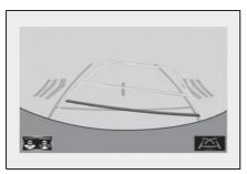
Example (Panoramic view monitor) (if equipped): Vehicles are approaching from both sides of the vehicle
