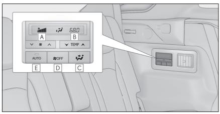
A djust the rear seats fan speed setting
