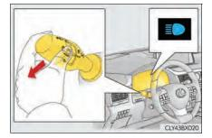
2 Press the Automatic High Beam switch.
