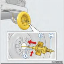
**8** Tilt the bracket (B) and pass it through the wheel opening. Then remove the hoist assembly (C).
