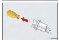
4 Install a new light bulb and then install the bulb base to the light unit by inserting it and turning it clockwise.
