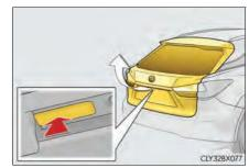
Pressing the switch while the power back door is opening/closing will stop the operation.
