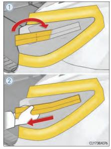
**5** Turn the bulb base counterclockwise and remove it.
