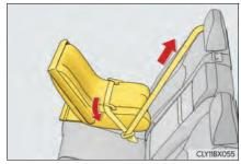
After installing the child restraint system, rock it back and forth to ensure that it is installed securely.  $(\rightarrow P. 66)$
