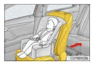
If the head restraint interferes with the installation of the child restraint system, and the head restraint can be removed, remove the head restraint.
