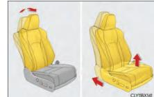
If the head restraint cannot be removed, raise it to the uppermost position.
