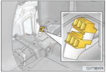
Remove the deck board and side auxiliary box cover and 12-volt battery cover.  $(\rightarrow P. 606)$
