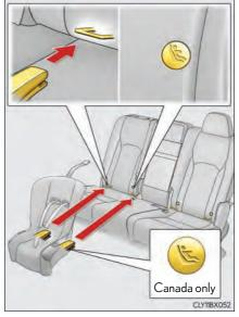
5 If the child restraint has a top tether strap, follow the child restraint manufacturer's operation manual regarding the installation, using the top tether strap to latch onto the top tether strap anchor.  $(\rightarrow P. 70)$
