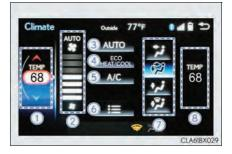
If the indicator is turned off, the system will blow ambient temperature air or heated air.
