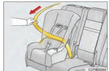
While pushing the child restraint system into the rear seat, allow the shoulder belt to retract until the child restraint system is securely in place.
