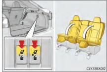
2 Check that the plate of the seat belt is on the front side of the seatback.
