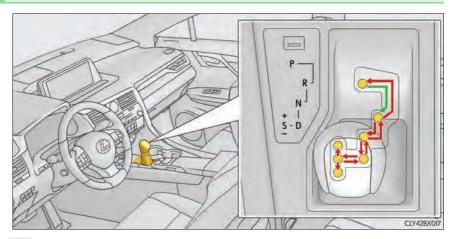
While the power switch is in ON mode, move the shift lever with the brake pedal depressed.
