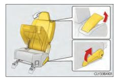
2 Pull the seatback folding lever and fold the seatback.
