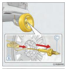
(A) and install the bracket (B) to the hoist assembly (C).
