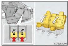
When using the seatback angle adjustment switch: If the rear seatback is reclined, adjust it to the most upright position and then press the switch again.
