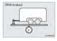
Additional optional equipment, passengers and cargo in the vehicle will reduce the trailer weight rating so as not to exceed GCWR, GVWR and GAWR.
