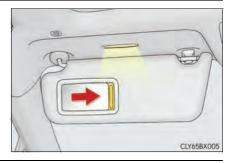
If the vanity lights remain on when the power switch is turned off, the light will go off automatically after 20 minutes.
