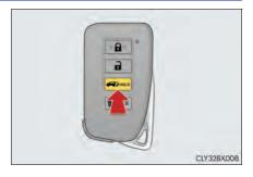
\*: Opening of the power back door when it is locked can be disabled by a customized setting. (→P. 741)
