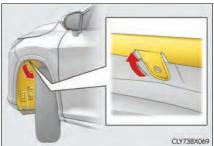
Partially remove the fender liner and turn the bulb base counterclockwise and remove it.
