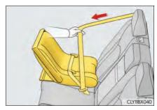
S While pushing the child restraint system down into the rear seat, allow the shoulder belt to retract until the child restraint system is securely in place.
