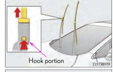
3 While disengaging the cap lock, using a tool such as a flathead screwdriver if necessary, remove the wiper insert.
