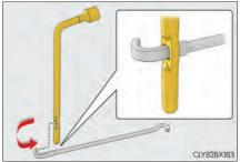
**5** Connect the jack handle to the adapter socket. Turn the jack handle counterclockwise.
