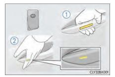
2 Touch the lock sensor (indentation on the surface of the door handle) to lock all the doors.
