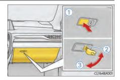
The glove box light turns on when the tail lights are on.
