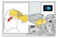
2 Press the Automatic High Beam switch.
