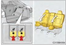
When using the rear seat operation switch (rear seat): If the rear seatback is reclined, bring the rear seatback to the most upright position and press and hold the switch again.
