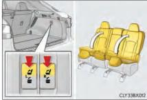
2 Check that the plate of the seat belt is on the front side of the seat.
