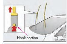
While disengaging the cap lock, using a tool such as a flathead screwdriver if necessary, remove the wiper insert.
