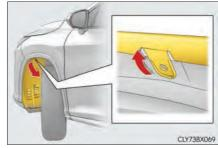
and turn the bulb base counterclockwise and remove it.
