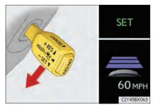
If the lever is operated while the vehicle speed is below approximately 30 mph (50 km/h) and a preceding vehicle is present, the set speed will be adjusted to approximately 30 mph (50 km/h).
