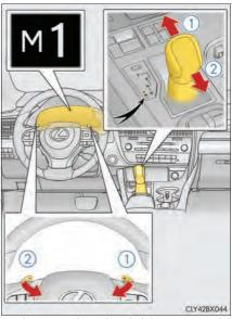
When in the M position, the gear will not change unless the shift lever or paddle shift switches are operated.
