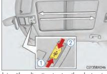
\*: Quickly slide and release the switch in either direction to stop the electronic sunshade partway.
