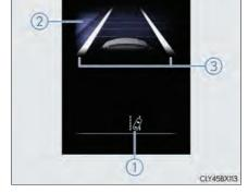
Indicates that steering wheel assistance of the steering assist function or lane centering function is operating.
