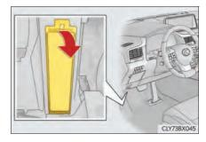
Remove the fuse with the pullout tool.
