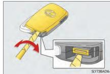
**3** Remove the depleted battery.
