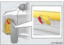
Partially remove the fender liner and turn the bulb base counterclockwise and remove it.
