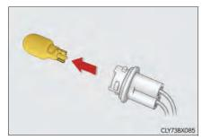
4 Install a new light bulb and then install the bulb base to the light unit by inserting it and turning it clockwise.
