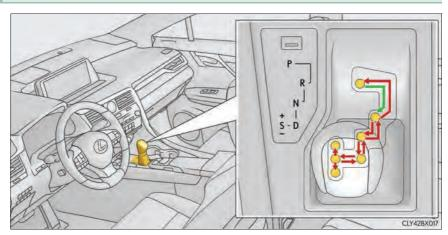
While the engine switch is in IGNITION ON mode, move the shift lever with the brake pedal depressed.
