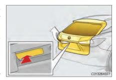
Pressing the switch while the power back door is opening/closing will stop the operation.
