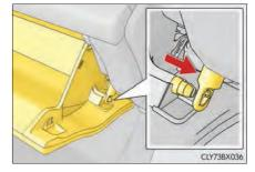
Push in the glove box on the vehicle's outer side to disconnect the claws. Then pull out the glove box and disconnect the lower claws.
