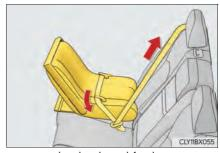
After installing the child restraint system, rock it back and forth to ensure that it is installed securely.  $(\rightarrow P. 68)$
