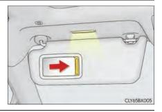
If the vanity lights remain on when the engine switch is turned off, the light will go off automatically after 20 minutes.
