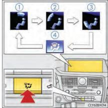
The air outlets used are switched each time the button is pressed.
