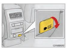
The power outlet can be used when the engine switch is in IGNITION ON mode.
