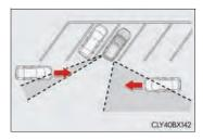
• Vehicles that the sensors cannot detect due to obstructions
