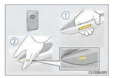
2 Touch the lock sensor (indentation on the surface of the door handle) to lock all the doors.
