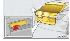
Pressing the switch while the power back door is opening/closing will stop the operation.
