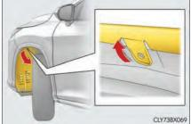
and turn the bulb base counterclockwise and remove it.
