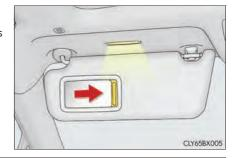
If the vanity lights remain on when the power switch is turned off, the light will go off automatically after  $20\,\text{minutes}.$
