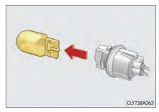
**5** Install a new light bulb and then install the bulb base to the light unit by inserting it and turning it clockwise.
