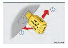
However, when a vehicle ahead is not detected, cruise control does not resume when the vehicle speed is approximately 25 mph (40 km/h) or less.
