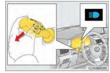
2 Press the Automatic High Beam switch.
