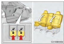
When using the rear seat operation switch (rear seat): If the rear seatback is reclined, bring the rear seatback to the most upright position and press and hold the switch again.
