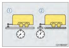
The gross trailer weight, gross axle weight and tongue weight can be measured with platform scales found at a highway weighing station, building supply company, trucking company, junk yard, etc.
