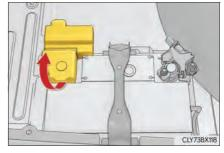
Remove the fuse with the pullout tool.
