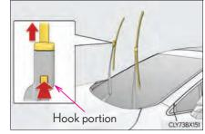
**3** While disengaging the cap lock, using a tool such as a flathead screwdriver if necessary, remove the wiper insert.
