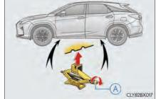
A Raise the vehicle until the tire is slightly raised off the ground.
