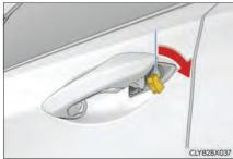
**3** Remove the key, return the handle, and then pull the handle again.
