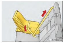
After installing the child restraint system, rock it back and forth to ensure that it is installed securely.  $(\rightarrow P. 70)$
