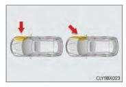
The SRS side airbags do not generally inflate if the vehicle is involved in a rear collision, if it rolls over, or if it is involved in a low-speed side or low-speed frontal collision.
