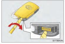
Remove the depleted battery.
