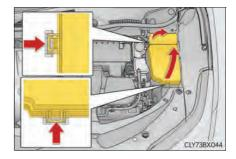
▶ Driver's side instrument panel Remove the lid.
