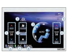
Select on the air conditioning control screen to display the option control screen. The functions can be switched on and off.
