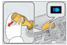
2 Press the Automatic High Beam switch.
