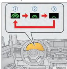
The pre-collision system is enabled and the system determines that the possibility of a frontal collision with a vehicle or pedestrian is high.
