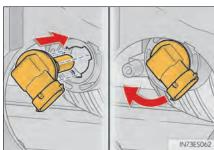
Shake the bulb base gently to check that it is not loose, turn the headlight high beams on once and visually confirm that no light is leaking through the mounting.
