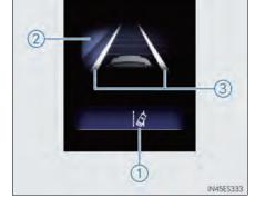
Indicates that steering wheel assistance of the steering control function is operating.
