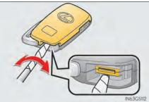
Remove the depleted battery.
