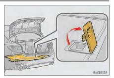
**2** The lever can be hooked on the edge of the trunk.
