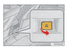
The power outlets can be used when the engine switch is in ACCESSORY or IGNITION  $\ensuremath{\mathsf{ON}}$  mode.
