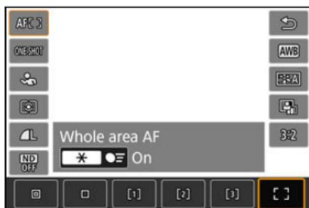
Uses auto selection AF in a whole-area AF frame to cover a larger area than Flexible Zone AF, which makes focusing easier than with 1-point AF/Flexible Zone AF and effective for moving subjects.
