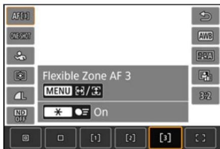
With Flexible Zone AF 1–3, you can freely set the size of the Zone AF frame (☞). Uses auto selection AF in Zone AF frames to cover a larger area, which makes focusing easier than with 1-point AF and effective for moving subjects. Focusing areas are determined not only based on the nearest subject but also based on a variety of other conditions such as faces (of people or animals), subject motion, and subject distance.
