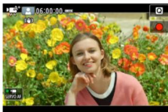
In [🌸<sup>A</sup>] recording mode, the camera detects the type of scene and sets all settings accordingly. The detected scene type is indicated in the upper left of the screen. For icon details, see [Scene Icons](#).
