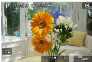
2. After the AF point in focus turns green, keep the shutter button pressed halfway and recompose the shot.
