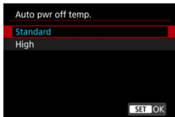
**[High]** sets the maximum temperature higher than the standard setting.
