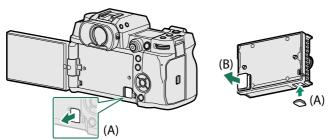
3 Place the fan on the camera, making sure the screws and connectors are correctly aligned.
