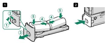
The batteries can be removed as shown.
