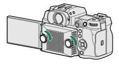
The cooling fan may fall off if the screws are not sufficiently tightened.
