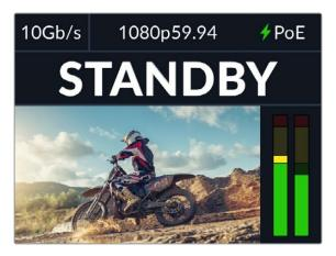
When power and video is connected, the PoE indicator will illuminate green, followed soon after by the video image and 'standby' indicator
