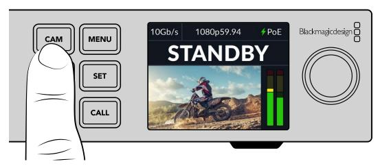
Press the camera, return 1 and return 2 buttons to check the camera signal and return feeds
