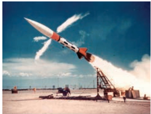
The HONEST JOHN was a simple, free-flight rocket capable of delivering a nuclear warhead. This highly mobile system was designed to fire like conventional artillery in battlefield areas. The Basic (M31) HONEST JOHN system was first deployed in 1954. It was replaced by the Improved (M50) HONEST JOHN in 1961, which reduced the system's weight, shortened its length, and increased its range. United States Army Photo.
