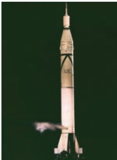
Juno 1 , a slightly modified Jupiter-C launch vehicle, shortly before the January 31, 1958, launch of America's first satellite, Explorer 1 . The Jupiter-C, developed by Dr. Wernher von Braun and the rocket team at Redstone Arsenal in Huntsville, Alabama, consisted of a modified version of the Redstone rocket's first stage and two upper stages of clustered Baby Sergeant rockets developed by the Jet Propulsion Laboratory. NASA.
