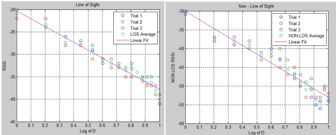
In the above plots, the distances are given in  $\log_{10}d$ , where  $d$  is in meters ranging from 1m to 10m. Three trails were performed and they are plotted together with their average and the linear fit curve.
