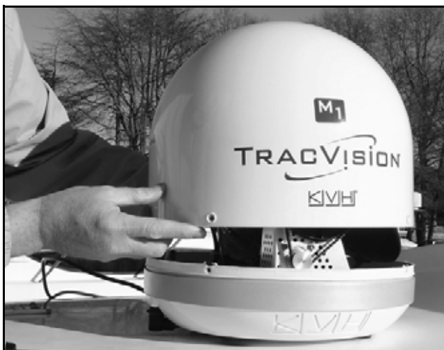
Figure 12: Removing the Radome
