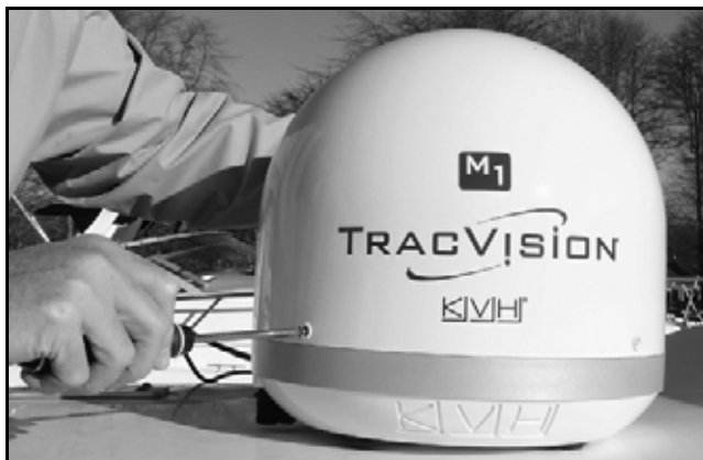
Figure 11: Removing the Radome Screws
