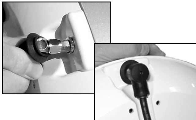
Figure 10: Protecting the Connector with the Rubber Boot
