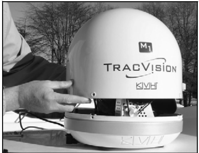
Figure 12: Removing the Radome
