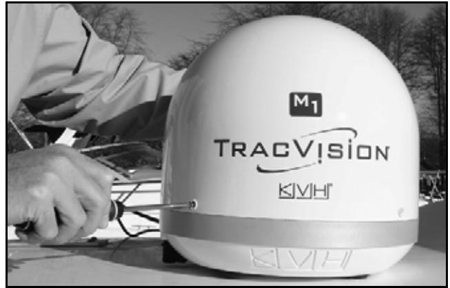
Figure 11: Removing the Radome Screws
