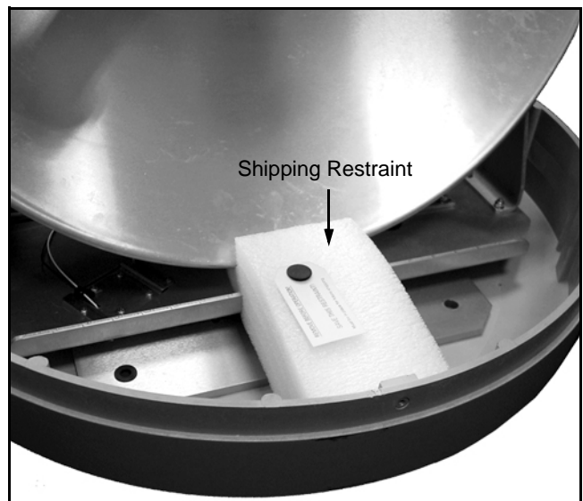
Figure 13: Foam Block Shipping Restraint
