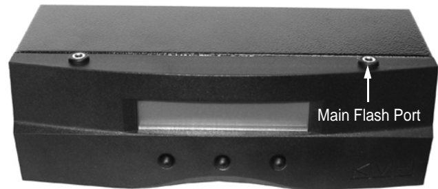
Figure 47: Main Flash Port on MCP
