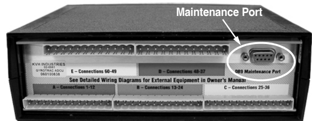
Figure 43: Maintenance Port on ADCU
