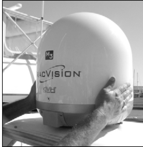
Figure 12 Removing the Radome
