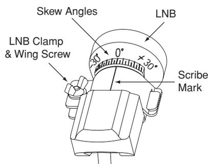
3. Carefully rotate the LNB so that the scribe mark on the LNB clamp is aligned with the proper angle measurement.
