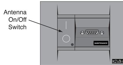
4. (*TracVision R5 only*) If the vehicle is moving, avoid turning the vehicle for 60 seconds after turning on the antenna to allow the antenna gyro to initialize properly.
