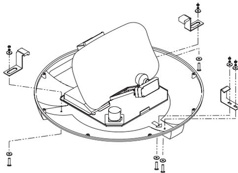
4. Place the antenna bracket on the forward shipping restraint.
