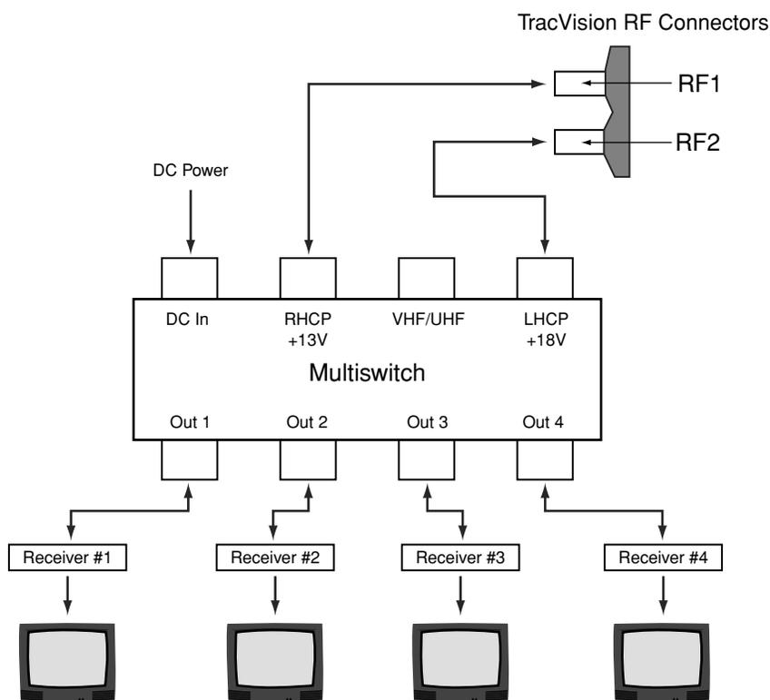
1. Connect the RF cable tagged "RF1" to the multiswitch input labeled "LNB RHCP +13V."
