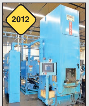
VERTICAL HYDRAULIC BROACHING MACHINE: Broaching Machine Specialties Mdl. Cell-Mate BMCM-1554 15-Ton X 54", S/N: 1762-12 (2012)
