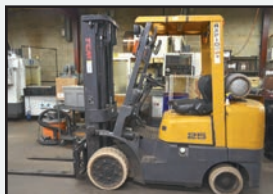
4,300-Lb. TCM Propane Operated Forklift Truck
