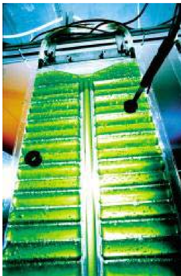
Figure 4.9 Algal Photobioreactor (Source: http://www.biopro.de/en/stern/magazin/01402/ )
