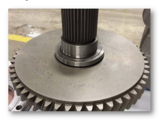
Make sure the lower gear is set the correct direction
