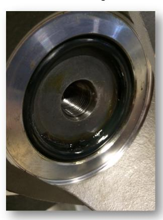
Attach o-ring plate and bolt
