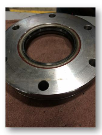
Install lower shaft cover plate o-ring
