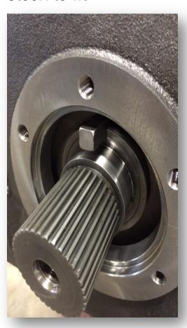
Drive in the key stock with a punch and insert snap ring
