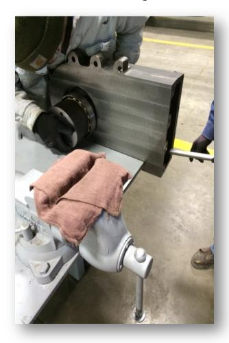
Drive lower shaft into case housing (use a soft hammer)
