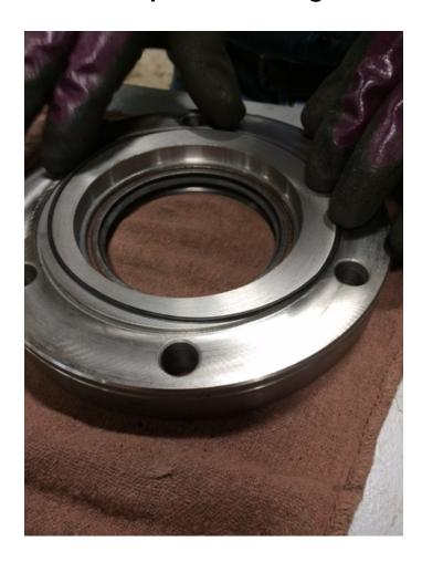
Apply grease to the lower shaft cover plate
