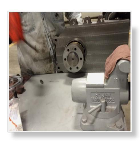
Fully seat the bearing to the gear box
