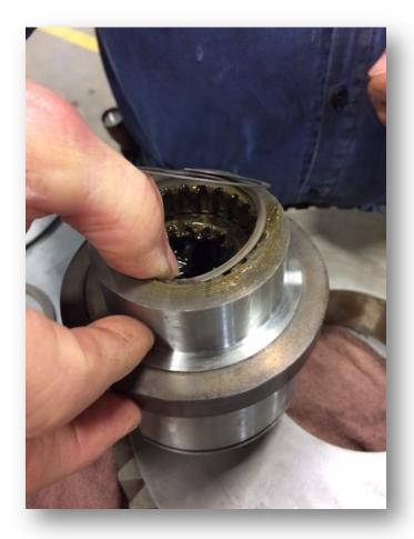
Apply lubricating oil to the gear coupler
