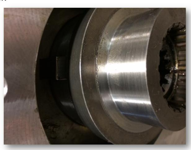
Slide the coupler housing through the gear and snap ring
