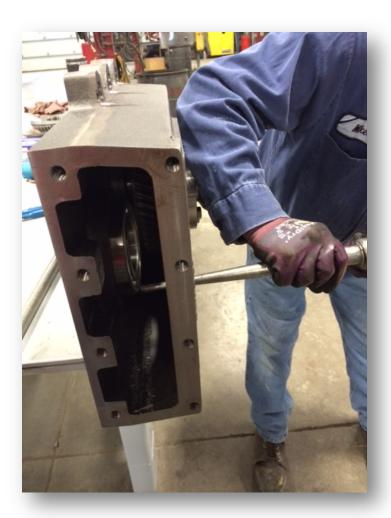
Place top gear in gear box. Note the left upper pitch to the gear direction
