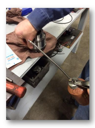
Insert coupler housing into gear and install key stock
