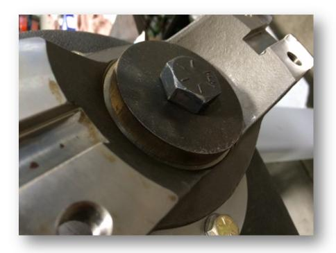
Install rear bearing in gearbox, if required
