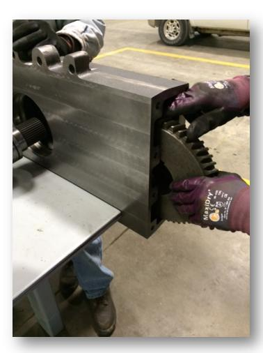
Use a small pry bar to align the shaft and gear
