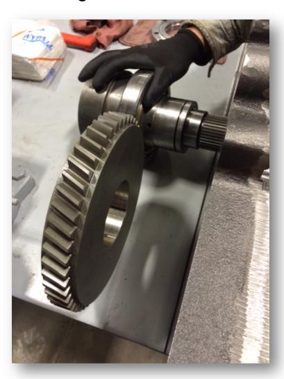
Insert lower shaft and push the shaft through the gear
