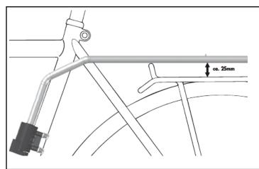
Position the bike seat so that the minimum distance between the bike seat frame and luggage rack, rear fender, or wheel is 25mm. The bike seat frame should be parallel to the ground. The load center (marked by a red point on your bike seat) may only be within 10cm behind the wheel hub. Please refer to your original bike seat manual for more information if needed.
