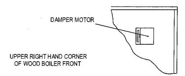
2. Attach the damper chain to the hole on the immediate left of the bottom hole in the motor wheel as shown below.
