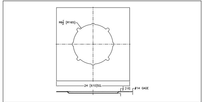
The roof sump receiver, also referred to as a bearing pan, is used when exact location of the drain can't be determined or when instances of opening the roof can not be precisely cut.
