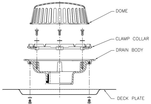
**Note:** Full installation is completed from the top of the roof deck, except for pipe connection.
