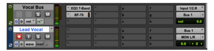
The Vocal Bus is getting input from the audio interface, and its output is into Bus 1. The Lead Vocal track is getting signal from Bus 1, and sending it to the stereo out of Pro Tools.
