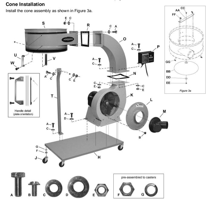
Figure 3: Assembly and hardware identification
