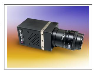
This InGaAs/GaAsSb type-II super lattice (T2SL) detector camera enables high resolution 1280x1024 SWIR imaging at frame rates at 90 frames per second (fps) at full resolution. The camera's small 12  $\mu$ m detector array pitch combined with the extended wavelength response of its T2SL material enables impressive imaging from visible wavelengths out to 2050 nm.
