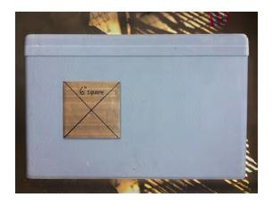
Cut a 6" square 4" from the left or right side and 4" from the bottom of the cooler (use a cardboard template to mark the cooler).
