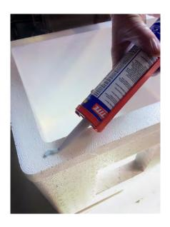
Seal the cooler using an adhesive such as Loctite PL 300 Foam Board Adhesive (fits caulk gun) of clear silicone sealant (such as GE II Window & Door Sealant) or hand-squeezable tubes of clear silicone sealant.
