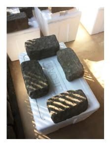
Weigh down the caulked cooler to allow sealant to fully dry (usually 24 hrs).
