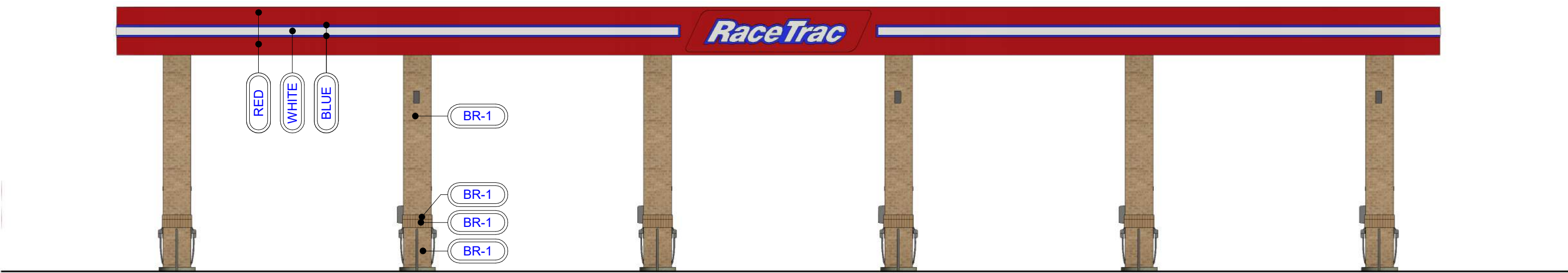
2 EDO CANOPY FRONT ELEVATION 1/8" = 1'-0"
