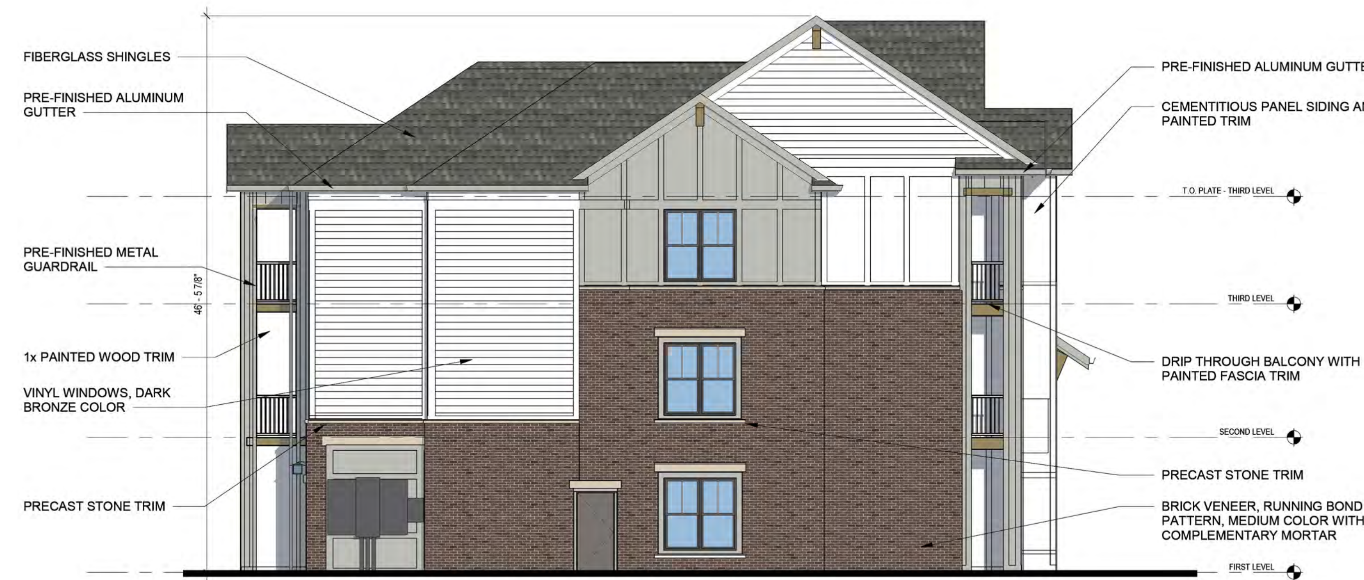
4 BLDG TYPE 1B - COLOR LEFT ELEVATION 1/8" = 1'-0"
