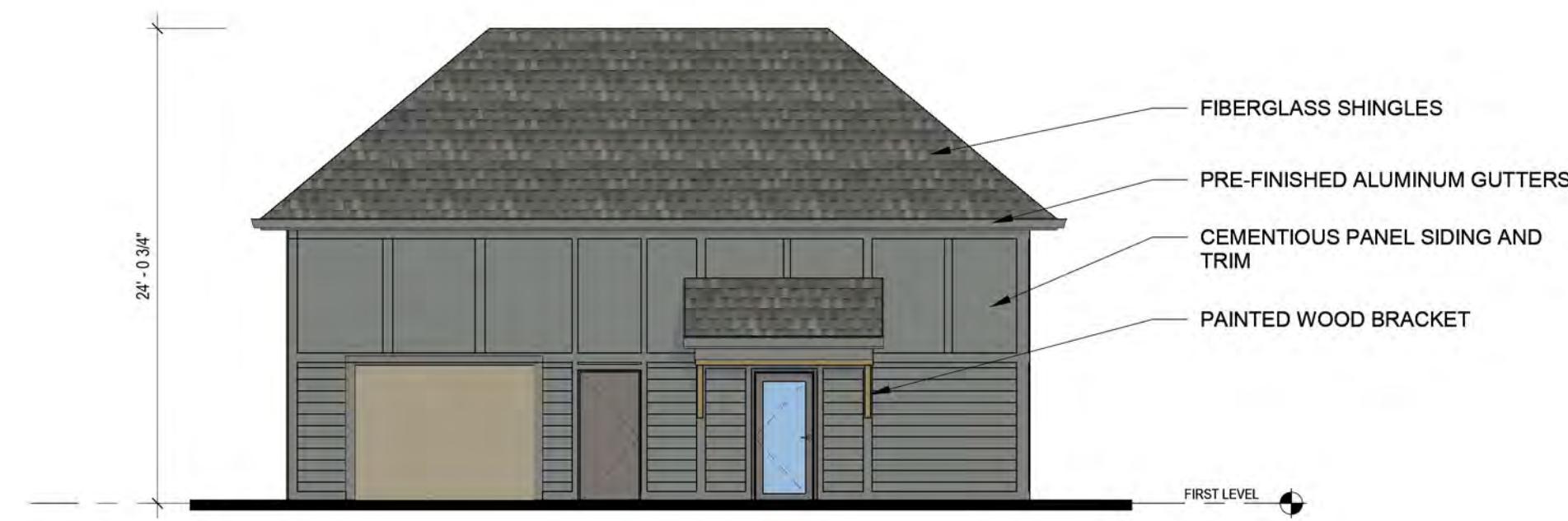
3 POOL HOUSE - SOUTH ELEVATION 1/8" = 1'-0" 0 8 16 24 32
