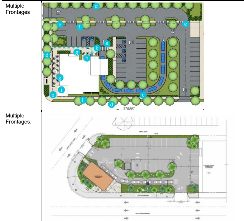
Example 4.1.D.3 Drive-through layouts. Note: Illustrative Examples below are meant to show general concepts and may not show required elements, such as bail out lanes.
