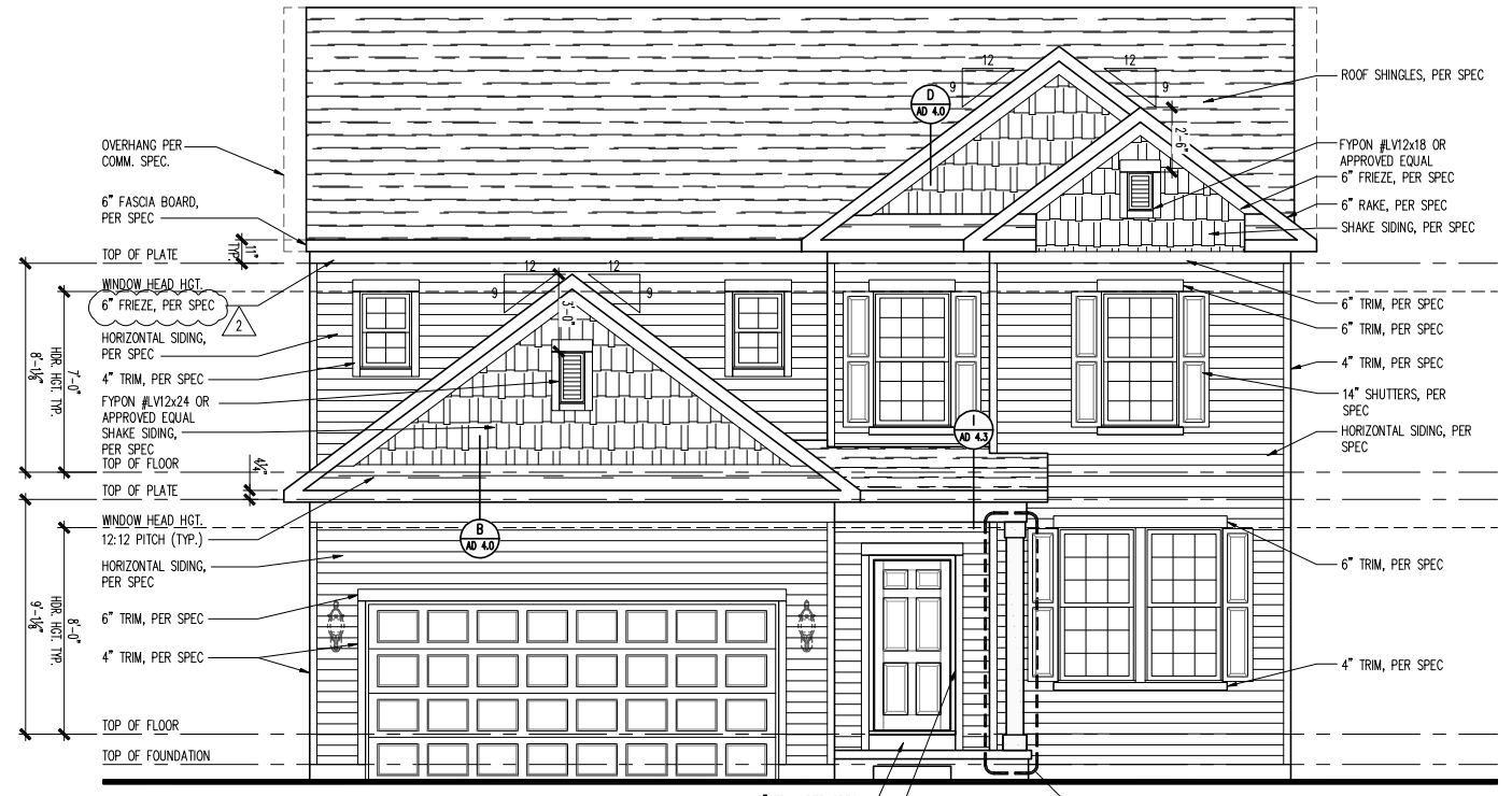
FRONT ELEVATION - HR102 SCALE: 1/4" = 1'-0"
