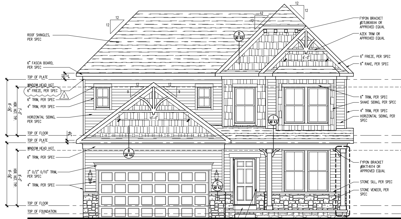
FRONT ELEVATION - QA301 SCALE: 1/4" = 1'-0"
