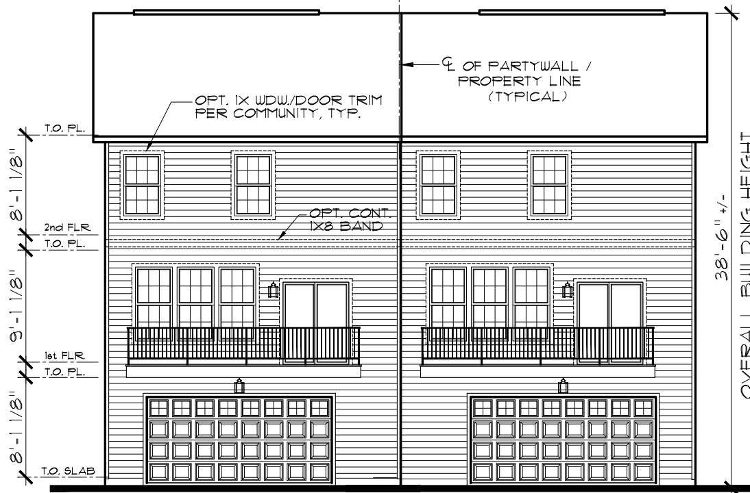
REAR ELEVATION 2-UNIT REAR-LOAD BUILDING
