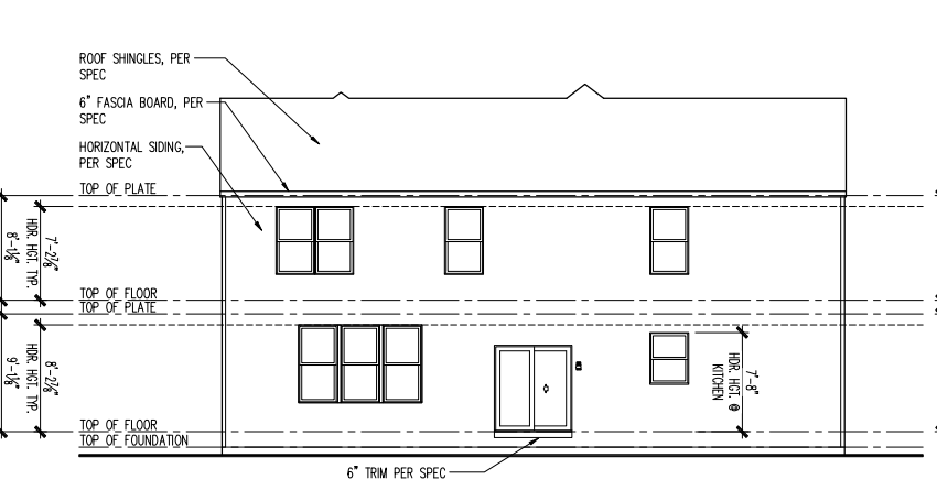
TYPICAL REAR ELEVATION SCALE: 1/8" = 1'-0"
