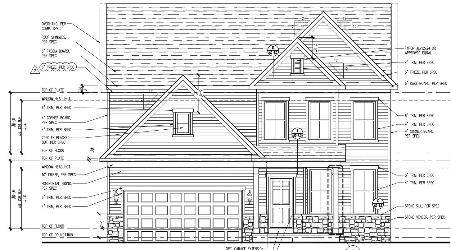
FRONT ELEVATION - LC201 SCALE: 1/4" = 1'-0"
