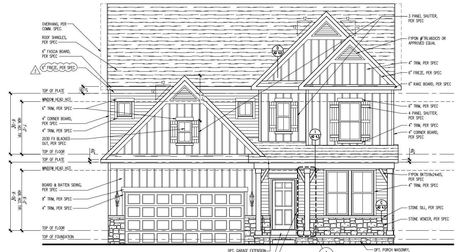
FRONT ELEVATION - FH201 SCALE: 1/4" = 1'-0"
