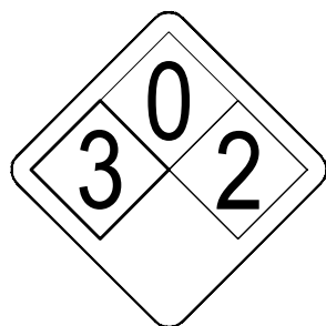
ALERTING SIGN (FOR CELL SITE BATTERIES)
