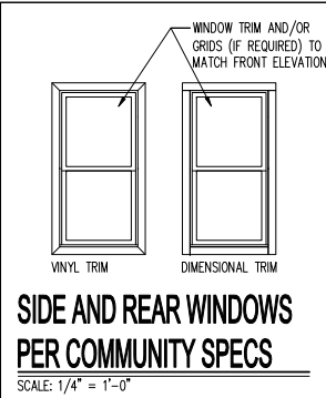
SIDE AND REAR WINDOWS PER COMMUNITY SPECS SCALE: 1/4" = 1'-0"
