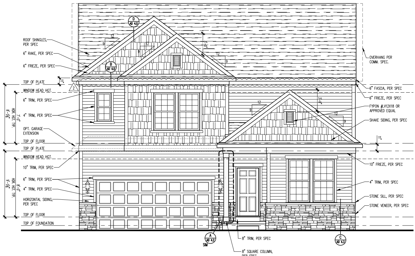
FRONT ELEVATION - HR201 SCALE: 1/4" = 1'-0"
