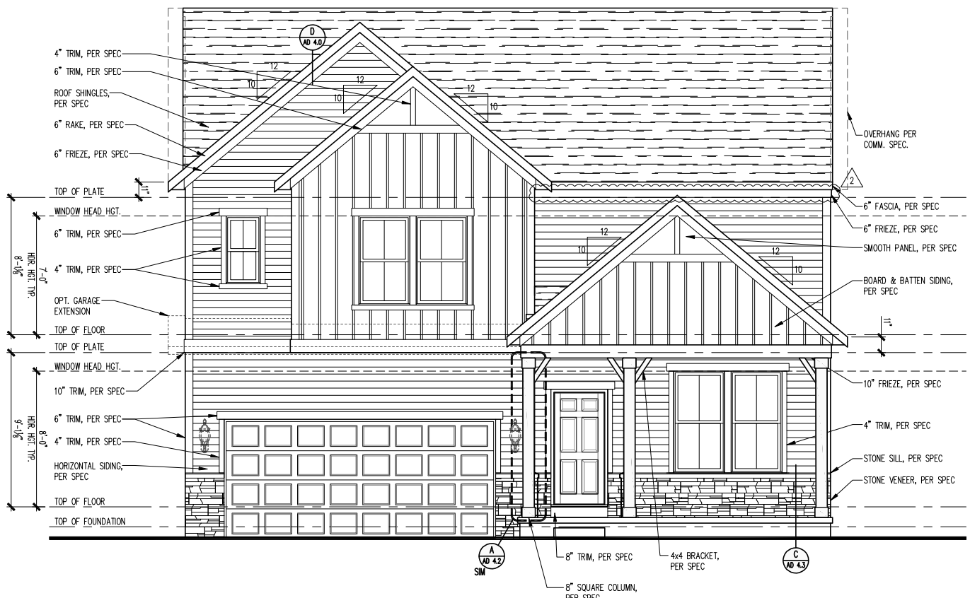
FRONT ELEVATION - FH101 SCALE: 1/4" = 1'-0"
