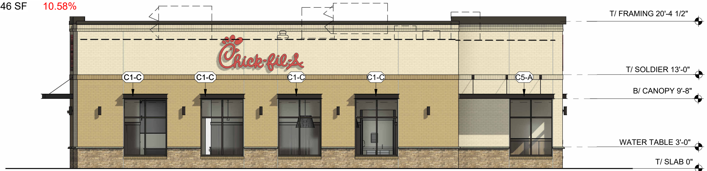
1 EXTERIOR ELEVATION (NORTH) 1/8" = 1'-0"
