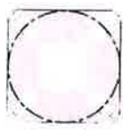
STL-1 Template 10.00 X 10.00 X 0.76 Anchor Plate 8.00-11.00" DIA. Bolt Circle
